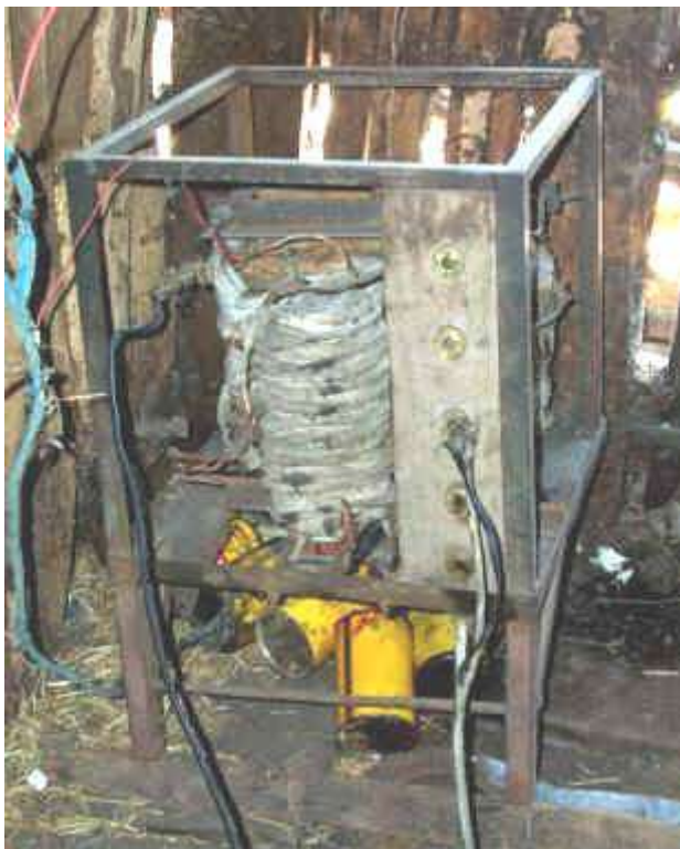
locally made welding machine
